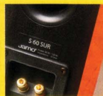
Simple single-wire 4mm terminals
